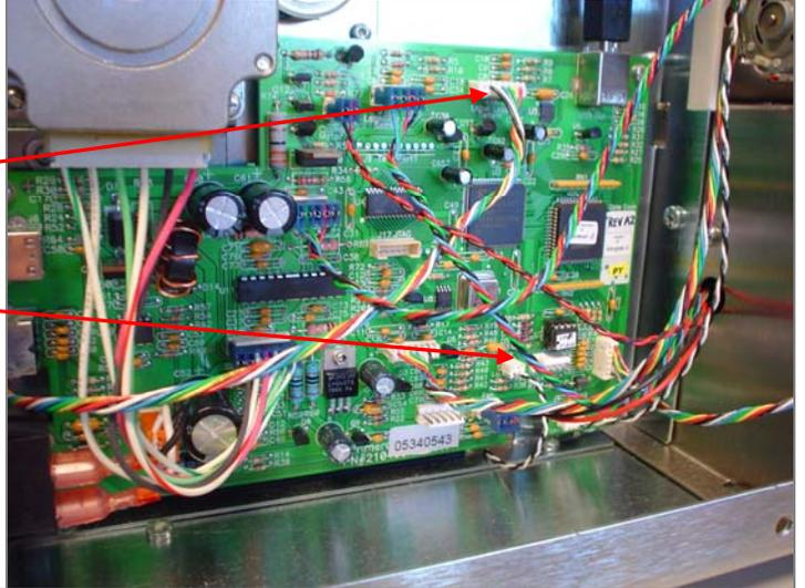
4. Remove two phillips screws securing the loop sensor bracket as shown.
