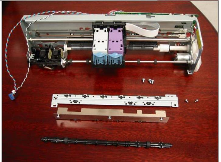
When replacing the print module take note of the screw and notched pins and the corresponding screw notch and tabs on both sides of the print module. **The tabs should be placed into the notched pins on both sides of the Print Module.**
