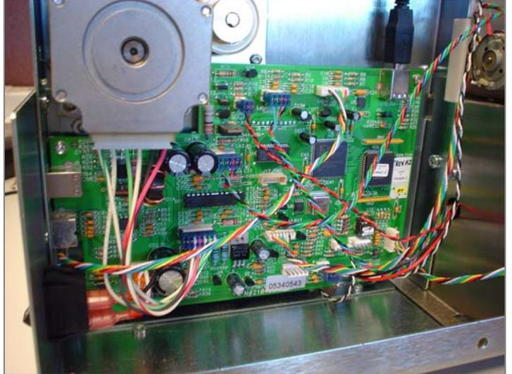
3. Remove the four T10 torx screws located at each corner of the main board.
