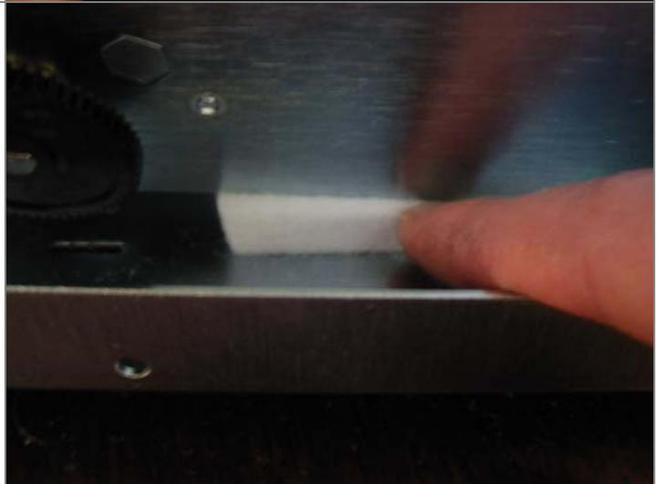
14. To complete the installation, snap the metal tabs under the metal roller guide.
