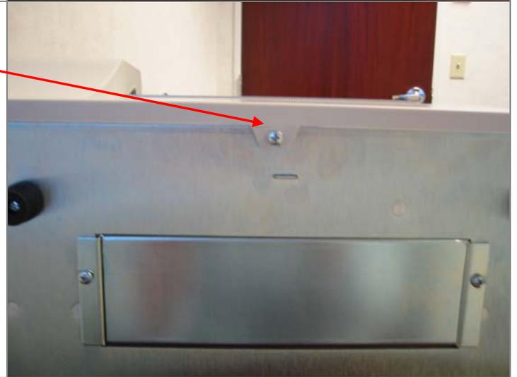
4. Loosen the top Phillips head screw which is attached to the Front Cover from behind.
